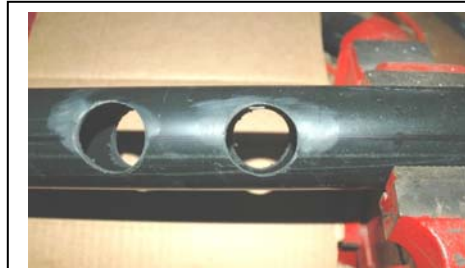
Figure 1A. Cut holes for side holes in pitfall covers.
