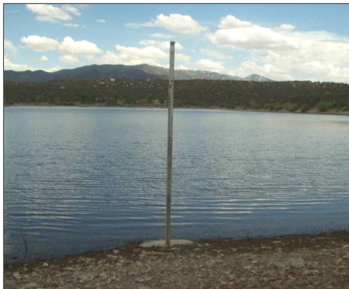
Figure 7.6 Photograph taken June 2006 of ineffective Parker Canyon Lake level gage.
