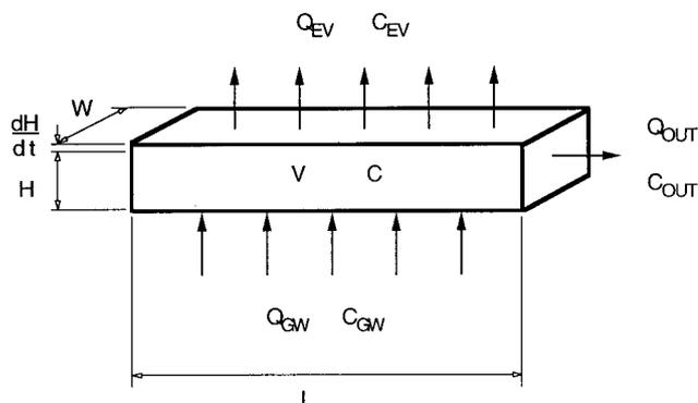
Figure 7. Control surface and boundary parameters for the conservative-tracer mass-balance model, where  $L$  is the channel length,  $W$  is the average channel width,  $H$  is the average water depth, and  $dH/dt$  is the change in depth over one time-step. Other terms are defined by Equations (1) and (2)
