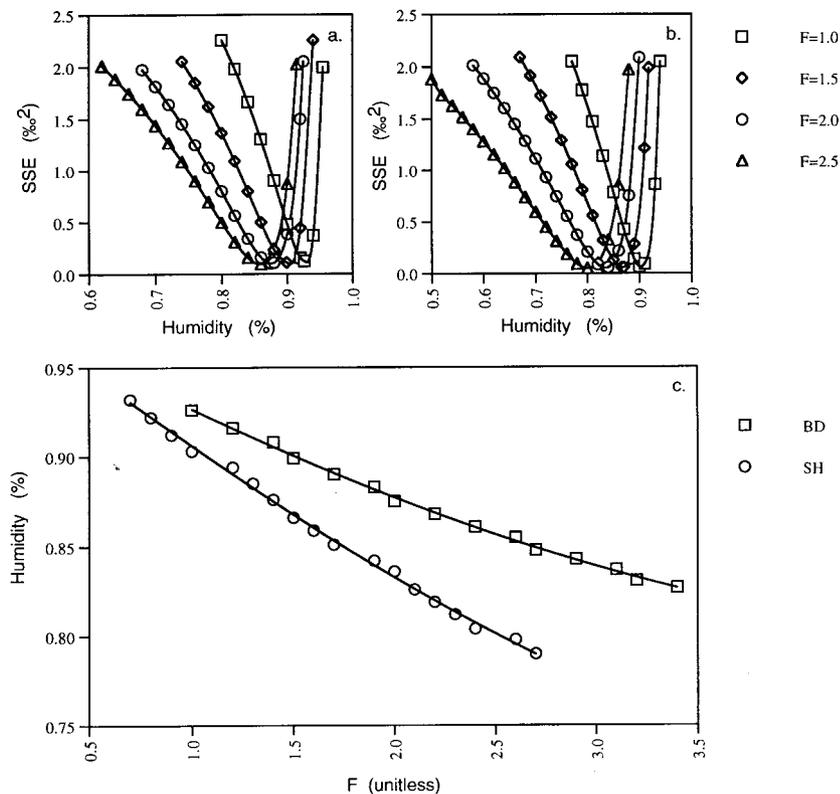
Figure 8. Mass-balance calibration data under recession conditions for stations BD (a) and SH (b), where SSE is the error square of sums (Equation 8) and  $F$  is the trial channel surface area divided by the initial estimate of channel surface area. The mass-balance model was solved by selecting trial values of  $F$ , varying humidity and computing SSE. Humidity and  $F$  combinations that produced SSE minima are plotted as the solution set of the models (c)
