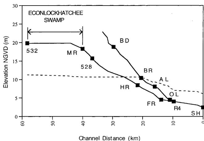
Figure 2. Channel elevations in the Big Econlockhatchee (lower solid line) and Little Econlockhatchee (upper solid line) Rivers. The potentiometric surface of the Floridan aquifer in the vicinity of the river is shown as a segmented line. Elevations are referenced to the national geodetic vertical datum (NGVD) (Sources: Wanielista *et al.*, 1992; Tibbals, 1990)
