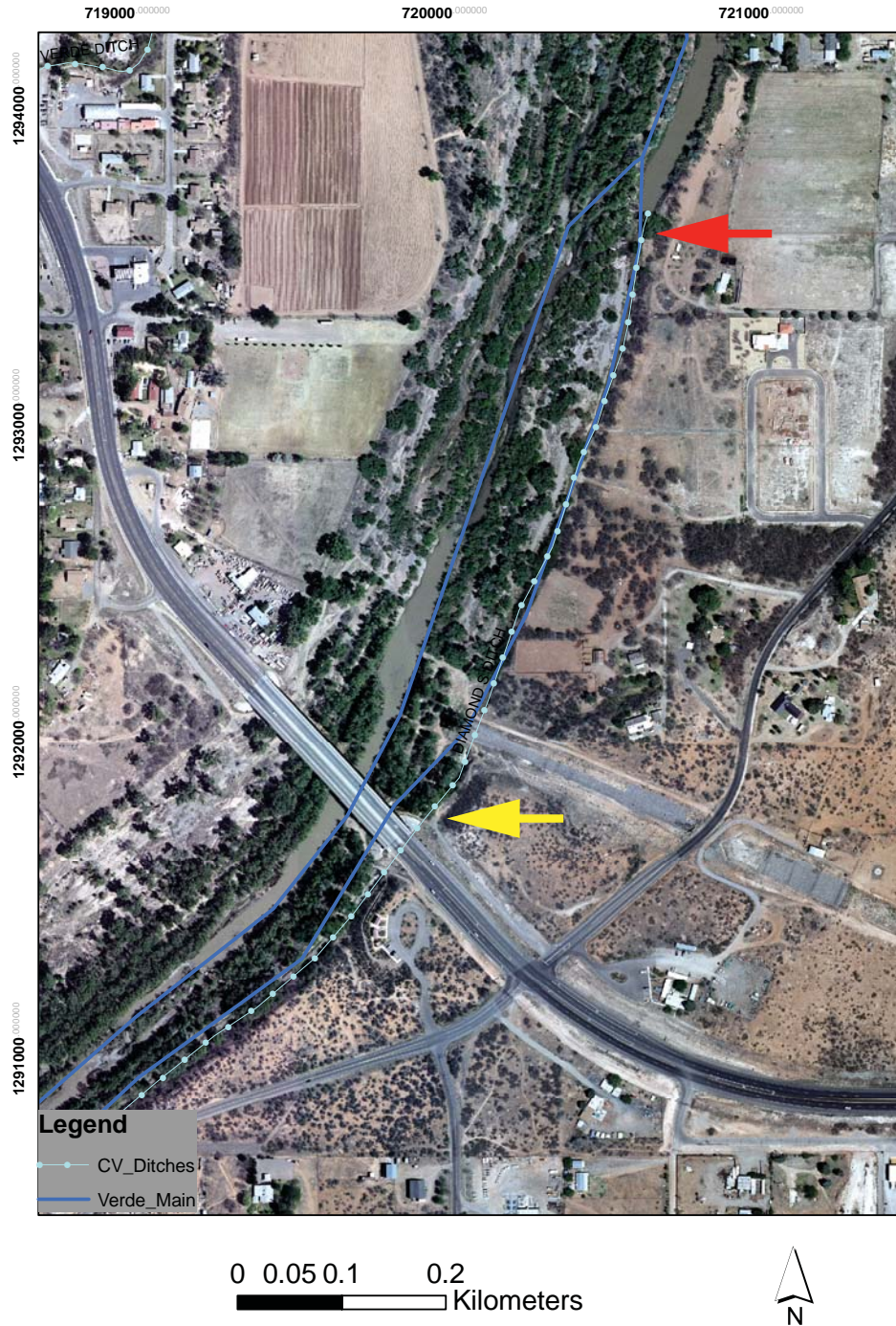
Figure 13 - Location of Diamond S Ditch diversion and head gates, Camp Verde, central Arizona. Red arrow is diversion structure, and yellow arrow is head gate structure. Initial spillway is directly above the head gates.
