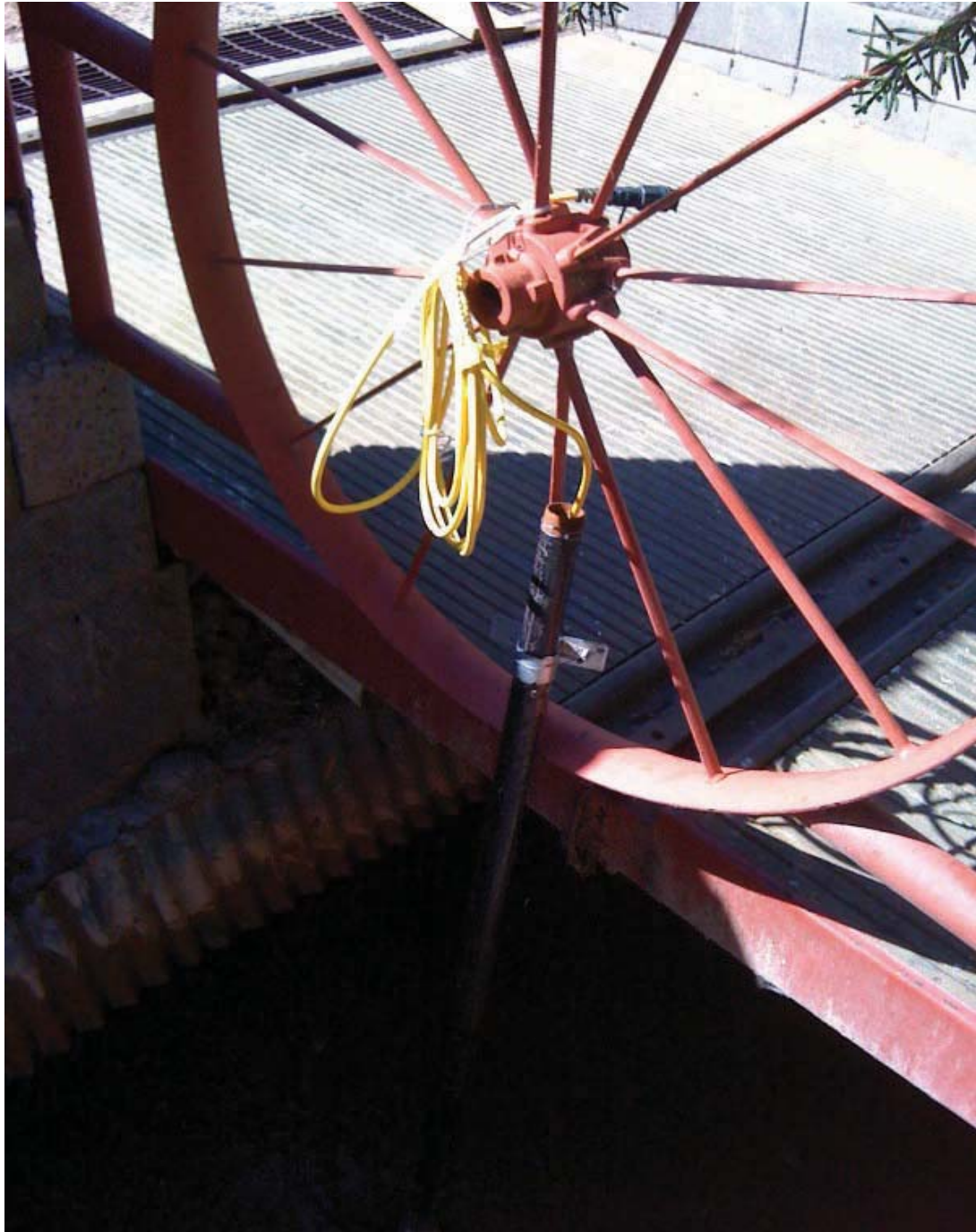
Figure 32 - Pressure transducer installed at Eureka Ditch return flow, Camp Verde, central Arizona. Shortly after this location, flow is returned to Beaver Creek.
