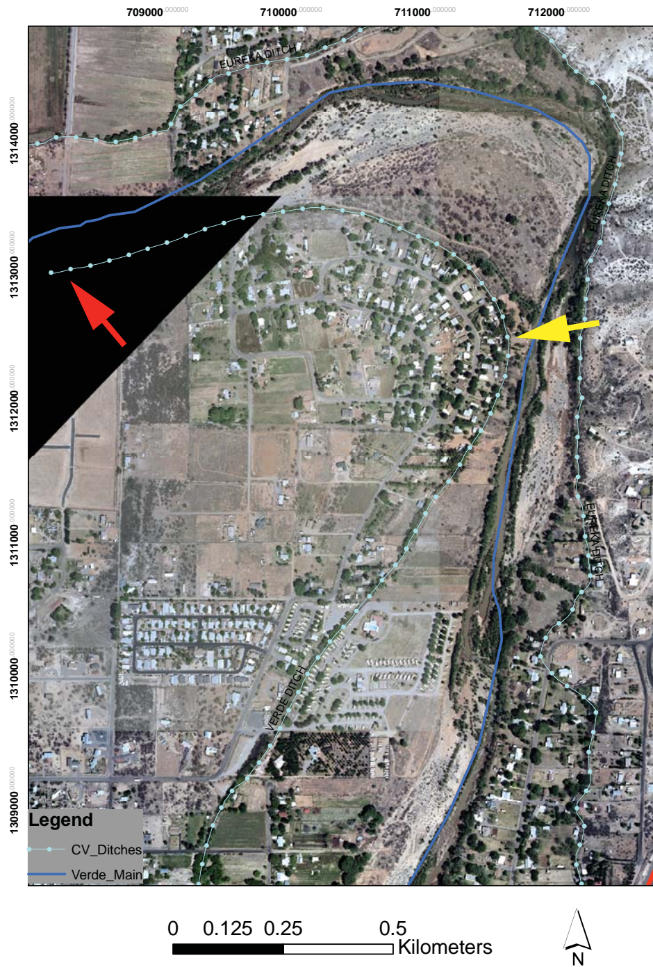
Figure 15 - Location map of the Verde Ditch diversion and head gates, Camp Verde, central Arizona. Red arrow is diversion structure, and yellow arrow is headgate. Large initial spillway is directly above head gate structure. Black triangle is gap in aerial photo coverage.
