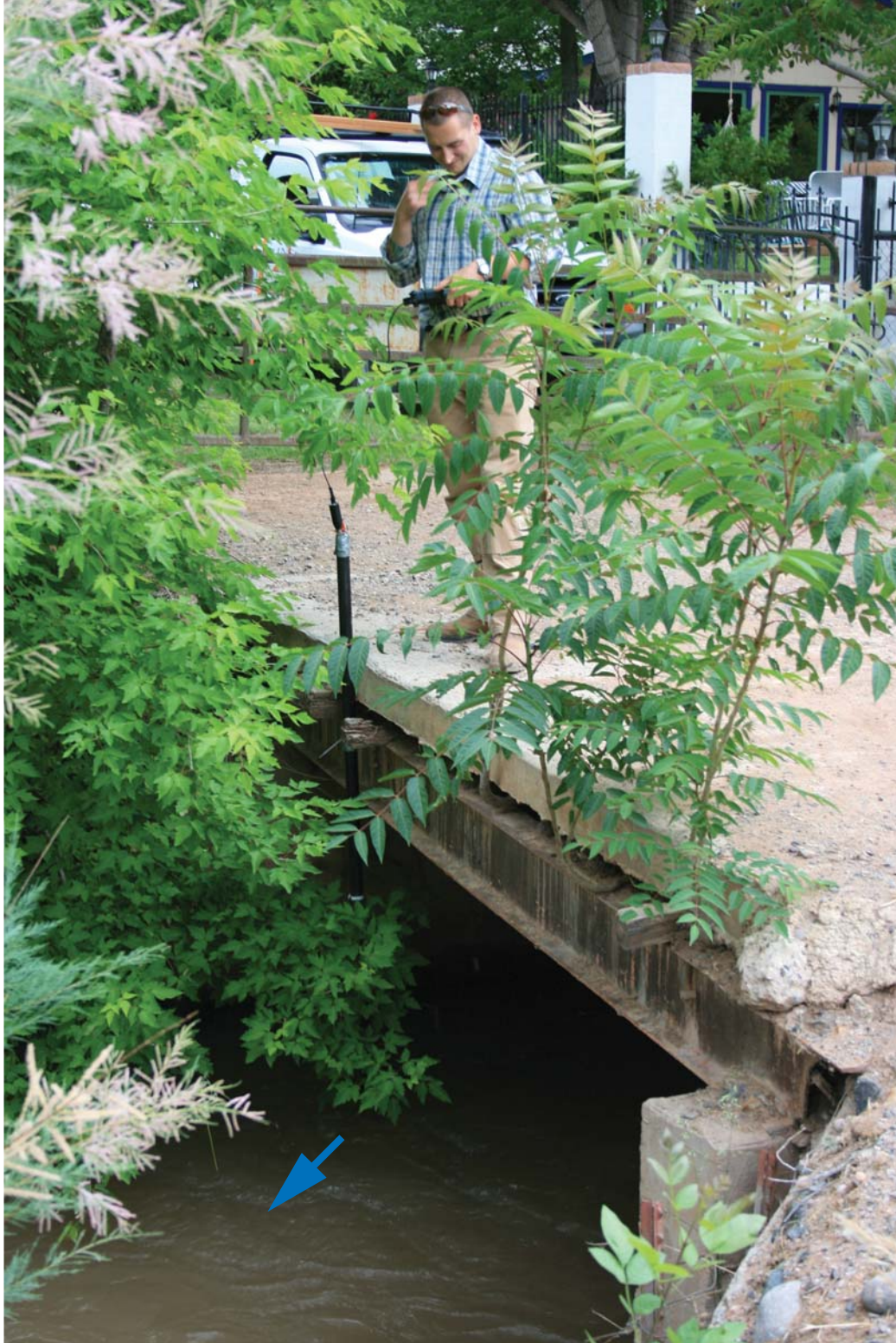
Figure 37 - Pressure transducer installed at Verde Ditch head gate prior to high-flow displacement, Camp Verde, central Arizona. Instrument was recovered after August 2009 floods and relocated to river left side of structure. Blue arrow indicates flow direction.
