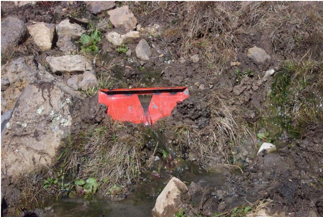
Figure 15 – Helocrene spring using a v-notch weir to measure discharge (Campbell Spring 2/22/03).
