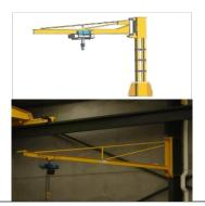
A type of crane where a horizontal member (jib or boom), supporting a moveable hoist, is fixed to a wall or to a floor-mounted pillar.
