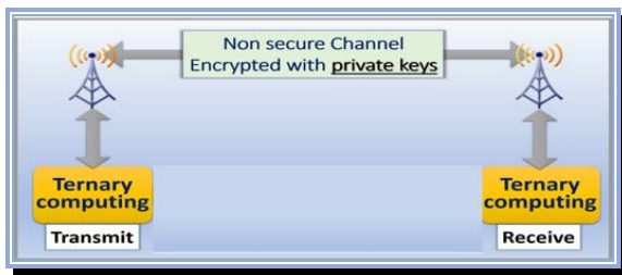
Fig. 2. Block diagram of ternary public keys to binary private keys exchange scheme
