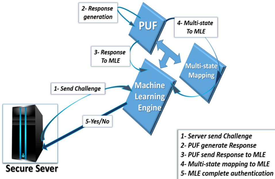
Fig. 4 Authentication protocol for memory-based PUFs with a machine learning engine (MLE)
