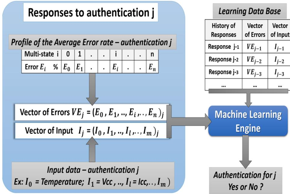
Fig. 3 CRPs error rates in multi-state PUFs
