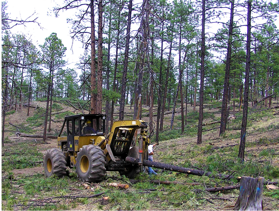
Using a skidder to remove small-diameter trees.
