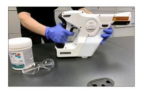
1. Removal of 32 oz. Tank. Rotate the dial of the tank lock towards the unlock position. Pull the tank release ring and carefully remove the tank. Hold on to the tank while pulling the ring or the tank may fall.<sup>1</sup>
