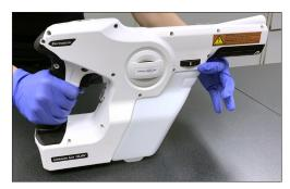
**3. Inserting tank back into sprayer.** Place the tank on a flat surface, and align the groves of the tank with the sprayer. Insert the tank into the sprayer until you hear the click of the release ring locking back into place. Rotate the dial of the tank lock towards the lock position to secure the tank in place.
