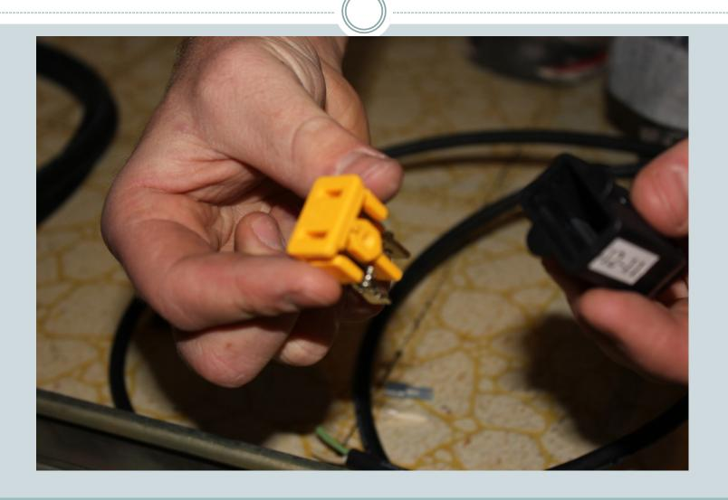
You may have to remove some rubber coating from the extension cord wires in order to connect it to the plug in.
