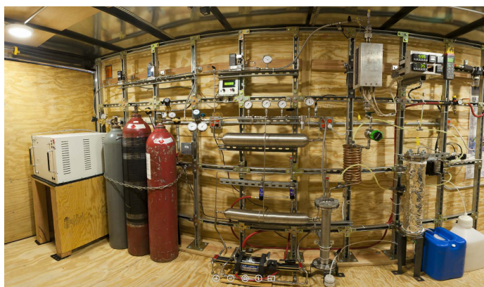
FIGURE 4. The fully assembled mobile MSU at NAU. Numbers correspond to major pieces of equipment: 1. Electrolyzer 2. Bottled synthesis gases 3. Low pressure buffer 4. Compressor 5. High pressure buffer 6. Methanol reactor/heating elements 7. Throttle valve 8. Condenser 9. Knockout drum 10. Distillation column. Red indicates high pressure ( 100bar) operation; yellow indicates low pressure ( 30bar) operation; gradients represent transitional pressure operation in the direction of the gradient. Not shown: pneumatic air compressor.
