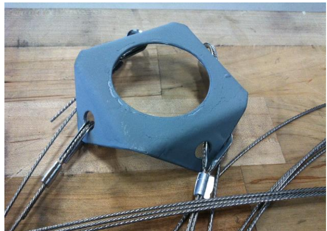
Figure 8: Guy Wire Fixture
