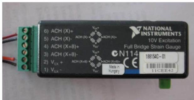
**Figure 23: NI SCC-SG Series Strain Gauge Input Module**
