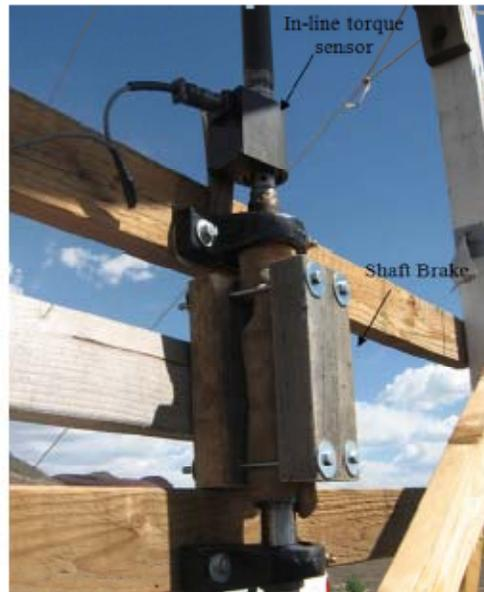
Figure 12: Experimental setup for Savonius rotor data collection.
