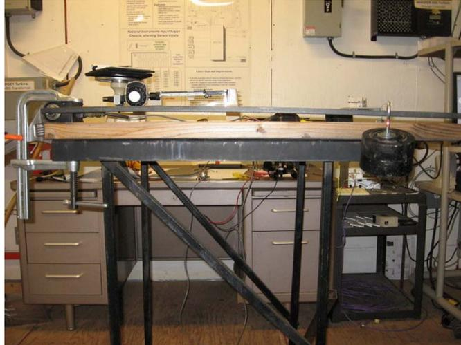
**Figure 24: Torque sensor calibration experimental setup**
