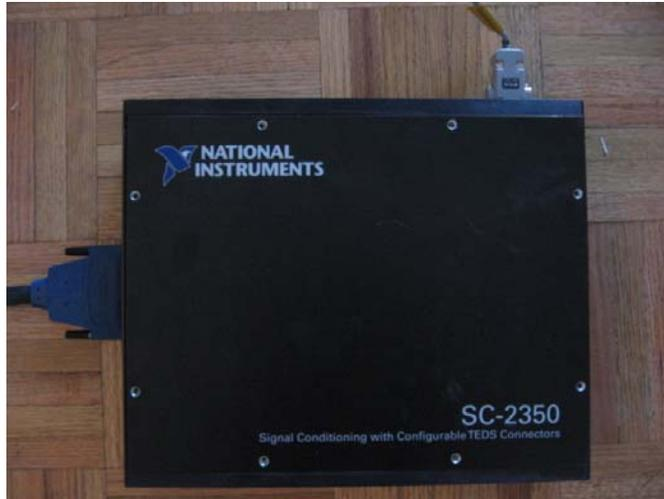
**Figure 18: NI SC-2350 Signal Conditioning**
