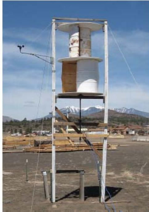
Figure 6: Example of a double-step Savonius rotor.
