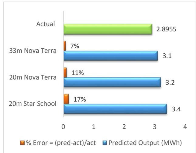
Fig. 1: Predicted annual energy output for Scharf turbine compared to actual annual energy output for April 2011 to March 2012
