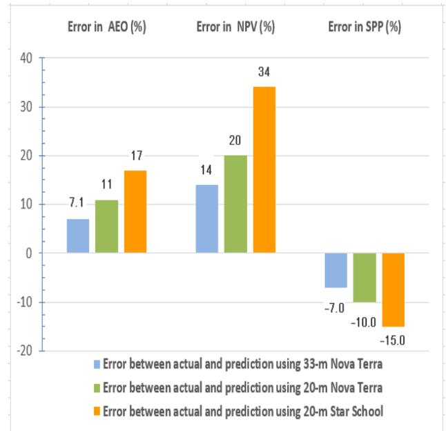
Fig. 3: Effect of errors in AEO to NPV and SPP
