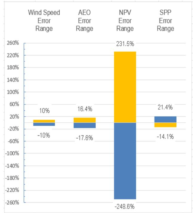
Fig. 2: Error ranges in AEO, NPV and SPP due to under- and over-predicted wind speed.
