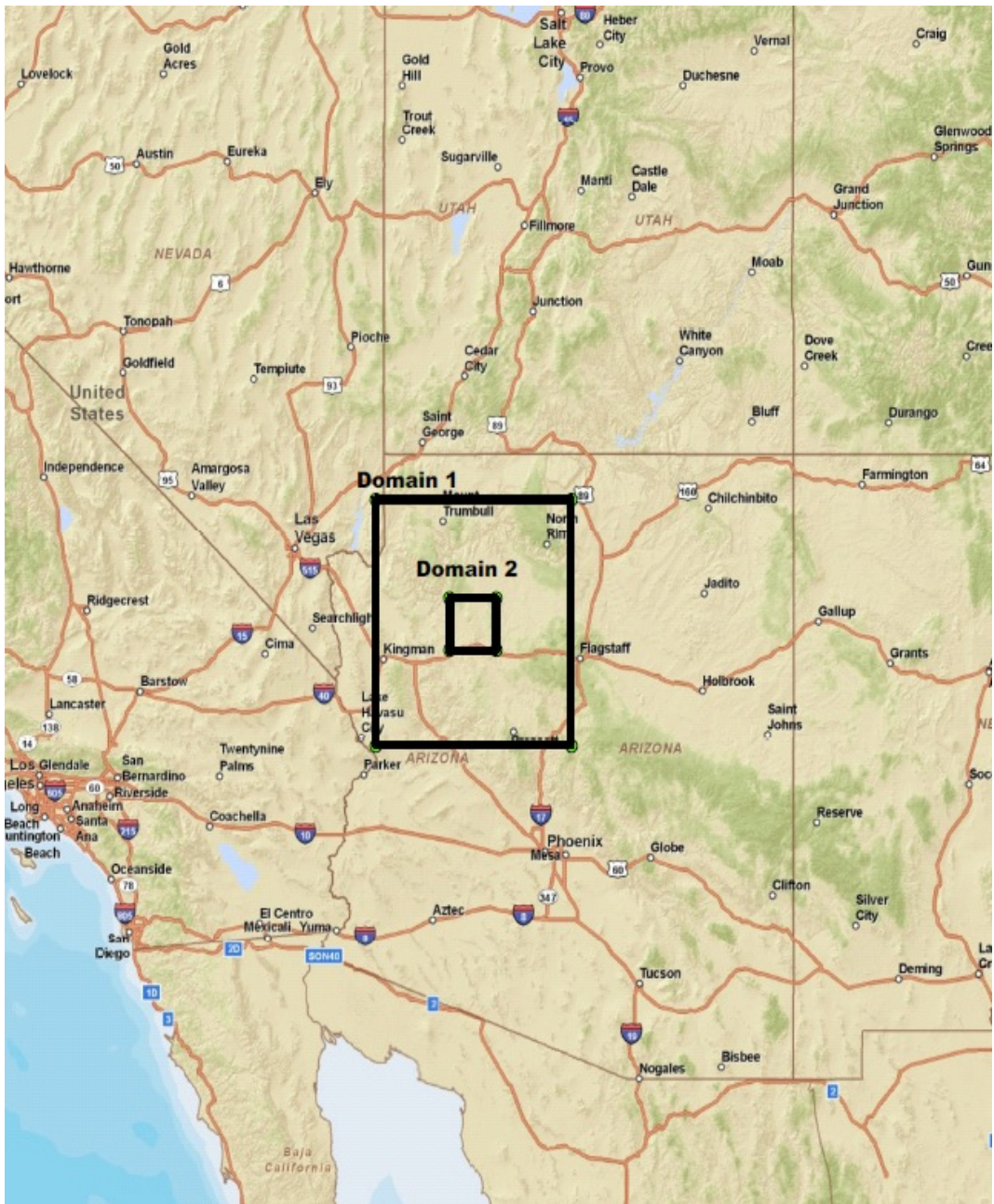
Figure 1: Representation of grid scheme A. Domain 1 corresponds to the outermost coarse domain with horizontal resolution of 3.0km and Domain 2 is the first nest domain with resolution of 1.0km.
