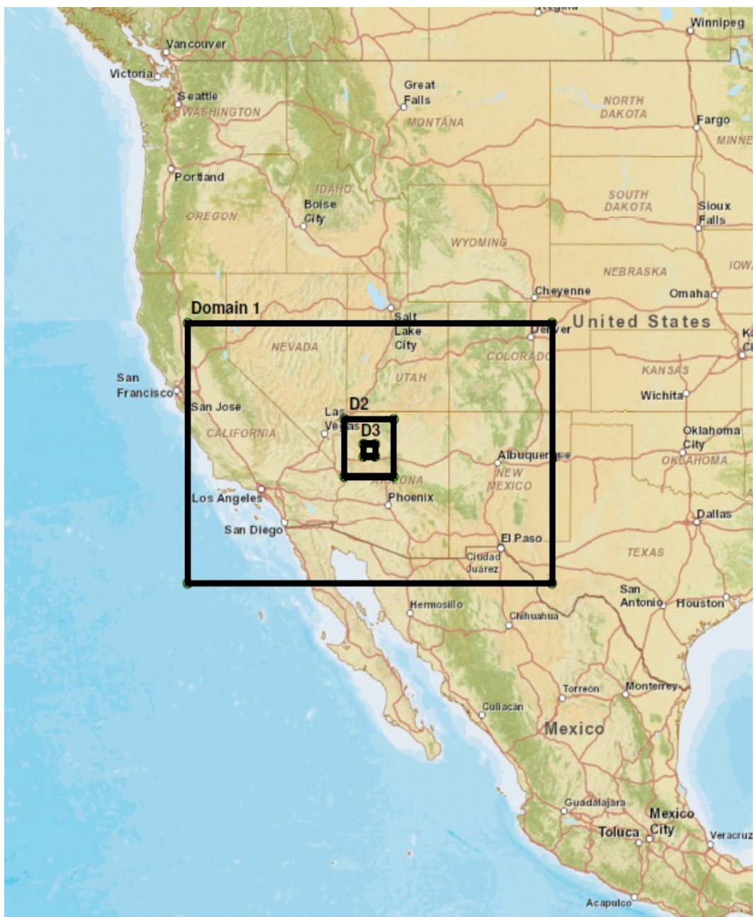
Figure 2: Representation of grid scheme B. Domain 1 corresponds to the outermost coarse domain with horizontal resolution of 9.0km, D02 is the first nest domain with resolution of 3.0km, and D03 is the second nested domain with resolution of 1.0km.
