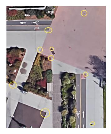
A list of coordinate values will be provided for control points and all other utility points collected as well as a comment/note of what the point is of (ex. 8" waterline bend) as well as include projection and datum information, specifically scale factor, datum, and spheroid/ellipsoid information. Preferably, the data is delivered in the following spatial reference system.
