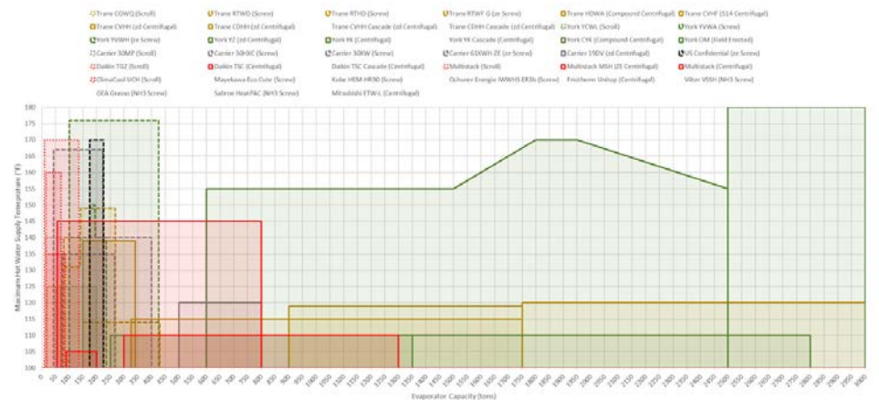
Figure 67. Available Heat Recovery Chillers for Different Design Conditions
