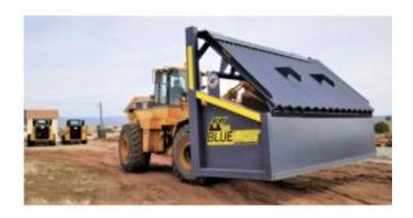
includes two different screening sizes to improve the operation of the composting process, contributing to the production of better quality compost.
