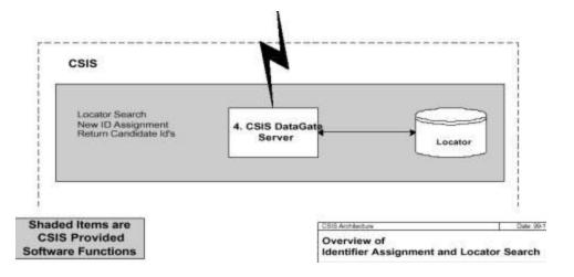
Figure.1 CSIS Architecture of System for Identifier Assignment and Locator Search (adopted from http://www.csis.k12.ca.us/library)
