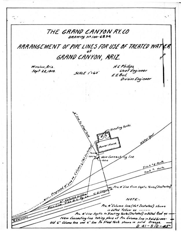
Figure 2: Grand Canyon Railway, "Arrangement of Pipe Lines for Use of Treated Water at Grand Canyon, Ariz.," Drawing No. 100-6894, 1909, GRCA 66101-28.
