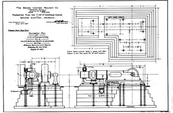
Figure 34: Foundation Plan for 11x18x14 Compound Engine, 1904, GRCA 30035AP.
