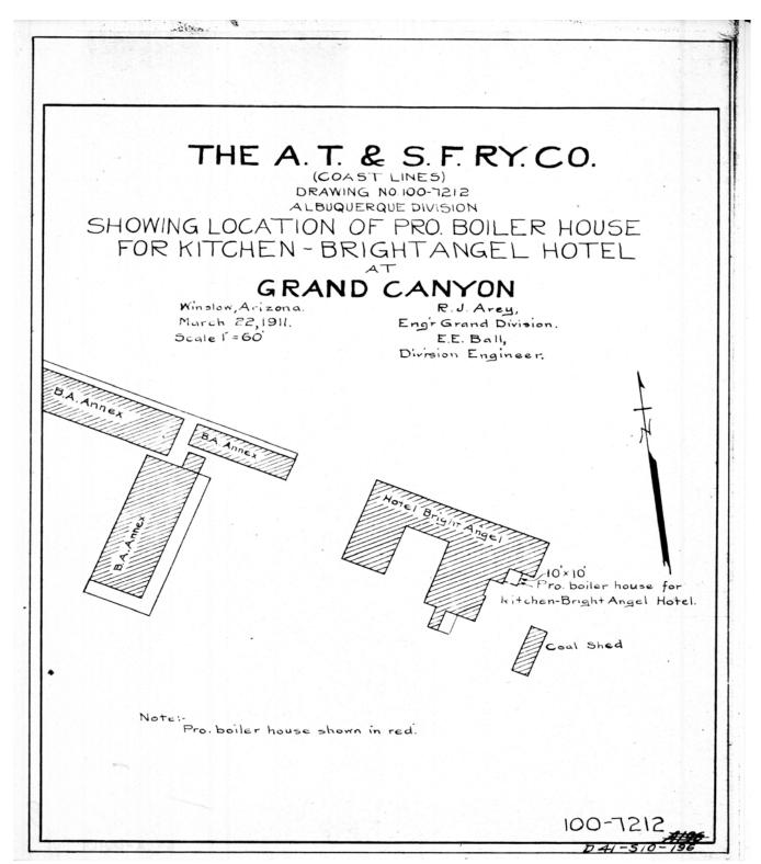
Figure 43: The AT&SF Ry Co., "Showing Location of Pro. Boiler House for Kitchen-Bright Angel Hotel at Grand Canyon," Drawing No. 100-7212, 1911, GRCA 66101-38.
