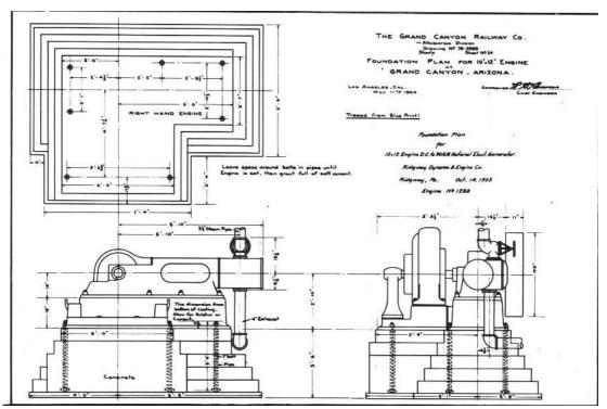
Figure 33: Foundation Plan for 10x12 Engine, 1904, GRCA 30035BC.
