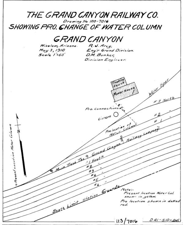
Figure 9: The Grand Canyon Railway Company, "Showing Pro. Change of Water Column, Grand Canyon," Drawing No. 100-7016, 1910, GRCA 34990.
