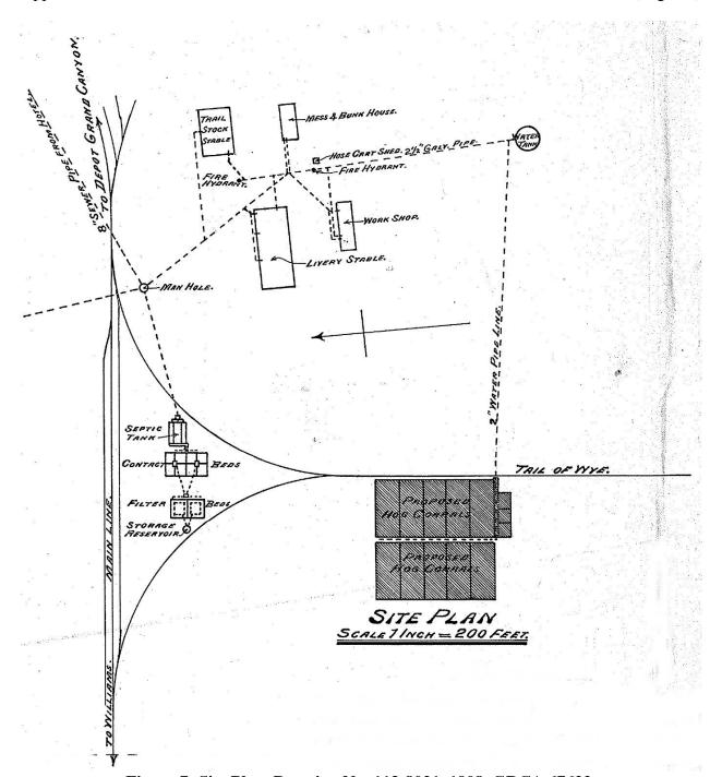
Figure 7: Site Plan, Drawing No. 113-8021, 1908, GRCA 67622.
