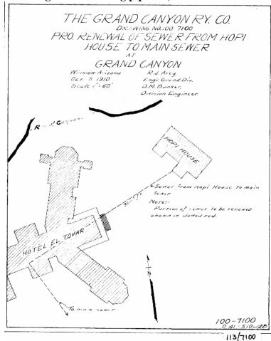
Figure 18: The Grand Canyon Railway Company, "Pro. Renewal of Sewer from Hopi House to Main Sewer at Grand Canyon," Drawing No. 100-7100, 1910, GRCA 66101-34.
