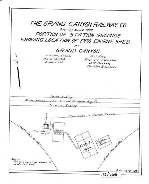
Figure 19: The Grand Canyon Railway Company, "Portion of Station Grounds Showing Location of Pro. Engine Shed, at Grand Canyon," Drawing No. 100-7008, 1910, GRCA 66101-30.
