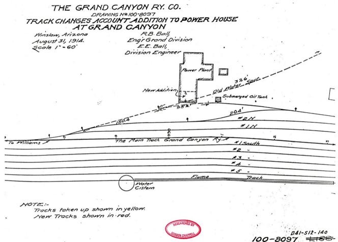
Figure 10: The Grand Canyon Railway Company, "Track Changes Account Addition to Power House at Grand Canyon," showing water cistern and flume track, Drawing No. 100-8097, 1914, GRCA 87923.
