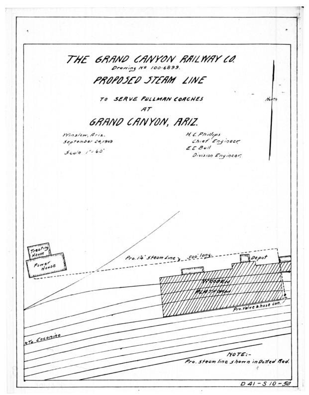
Figure 39: The Grand Canyon Railway Company, "Proposed Steam Line to serve Pullman Coaches at Grand Canyon, Ariz.," between Power Plant and Passenger Yard, Drawing No. 100-6899, 1909, GRCA 66101-29.
