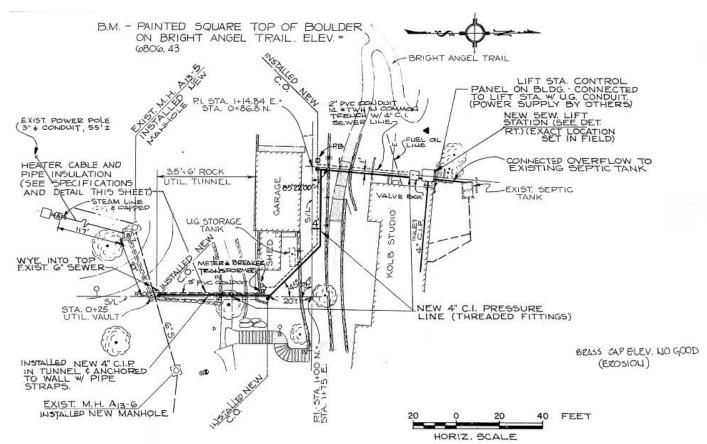
Figure 22: From 1973 existing conditions drawing for sewer system, p. 15, Drawing No. 113-41043A.
