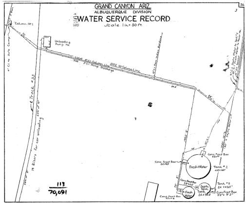
Figure 11: Water Service Record, showing pump house and three water tanks, Drawing No. 113-70091, Sheet 3.
