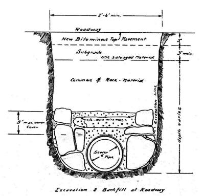
Figure 30: Sewer line construction detail, Drawing No. 113-5710, 1937.
