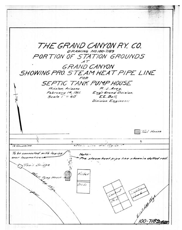
Figure 41: The Grand Canyon Railway Company, "Portion of Station Grounds at Grand Canyon Showing Pro. Steam Heat Pipe Line for Septic Tank Pump House," Drawing No. 100-7189, 1911, GRCA 66101-36.
