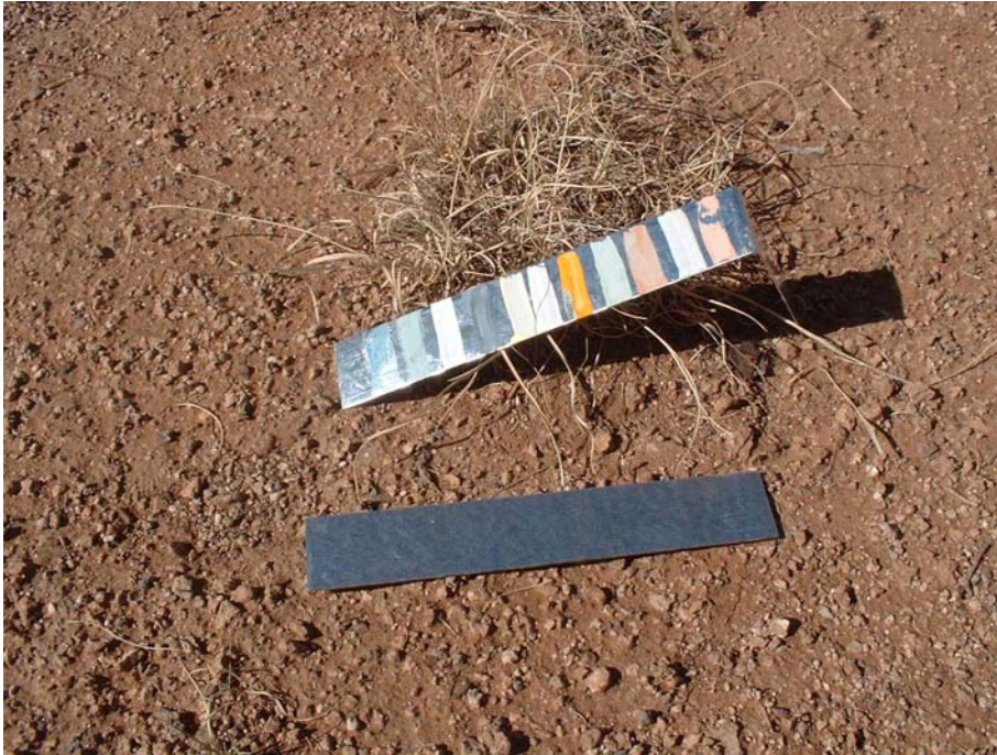
Figure 4. Pyrometer created with heat sensitive paint. The paint strips were arranged by temperature with the highest temperature closest to the bend in the metal. The pyrometer was covered with the strip of metal shown in the picture, attached with two small paperclips, and then pushed flush into the ground before the prescribed burn.
