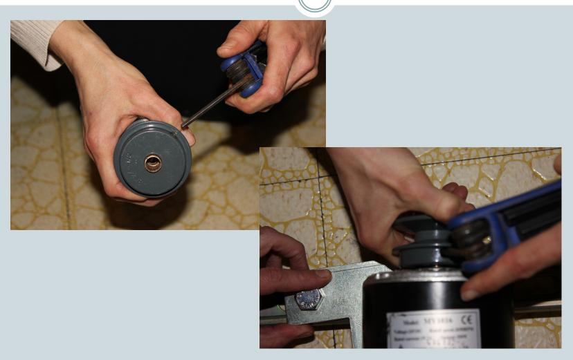
Adjust motor so that it is close enough to the bike that the v-belt will fit around the rear bike wheel and the belt pulley.
