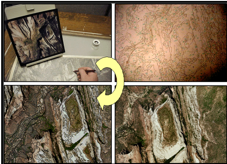
Figure 8. Example of transfer process from aerial 9 x 9 photography to color orthophoto base map.
